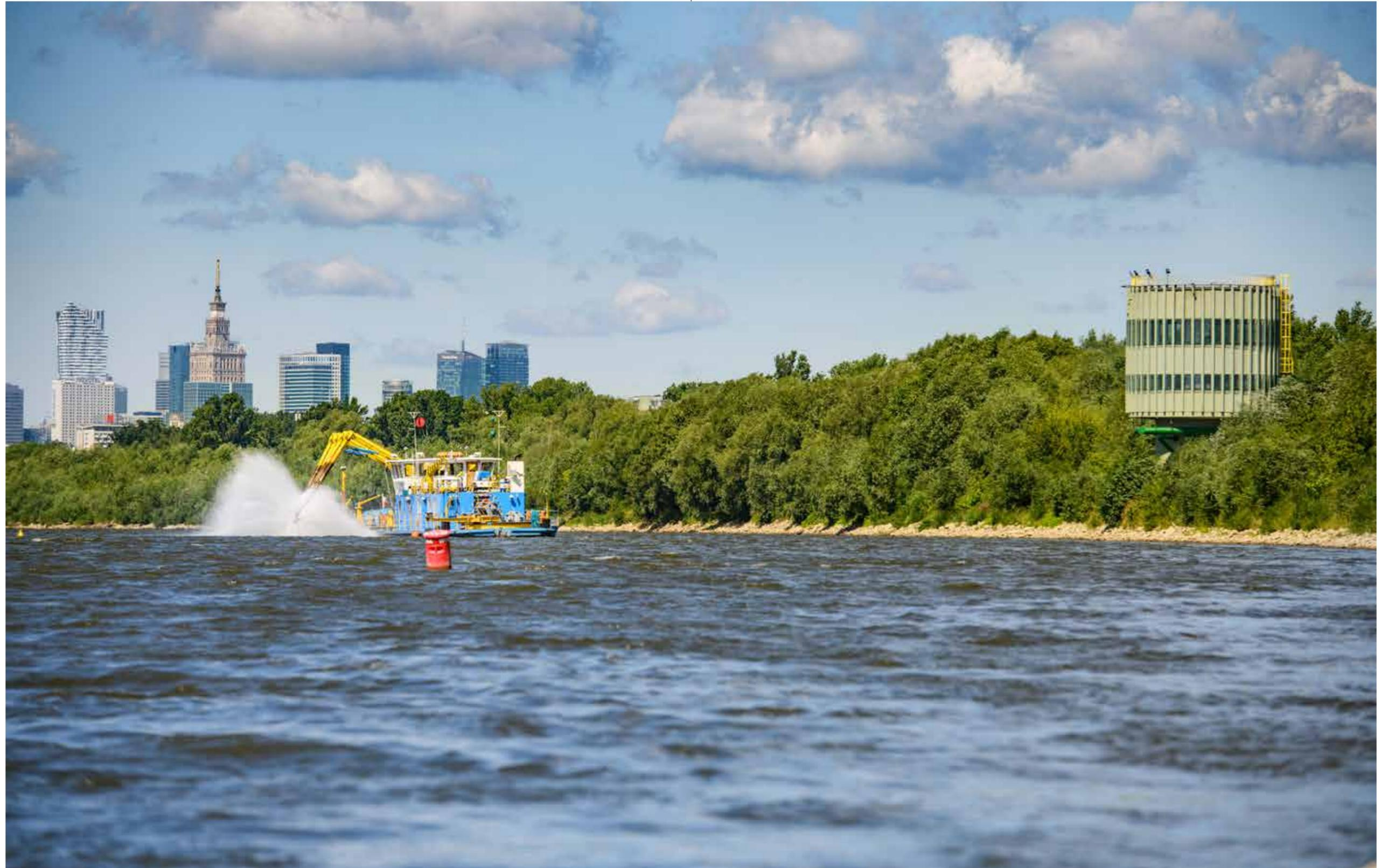
The "Chude Wojtki" hydraulic scarifiers, named after their creator – engineer Jerzy Wojtkowski, are specialised vessels. Their job is to flush the river bed with pressurised water to remove the top, most contaminated layer of sand. Pictured is one of the "Wojteks" at work on the Vistula River, photo by Jacek Turczyk
